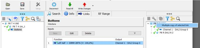
The window with confirmation appears. After confirmation, the sample link to the remaining receivers from the selected branch is automatically created. Then it is necessary to *Write changes* into devices. It is good to check and, if necessary, name the appropriate channels of the receivers correctly.
